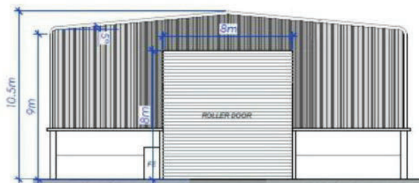
Figure 7: South West Elevation
