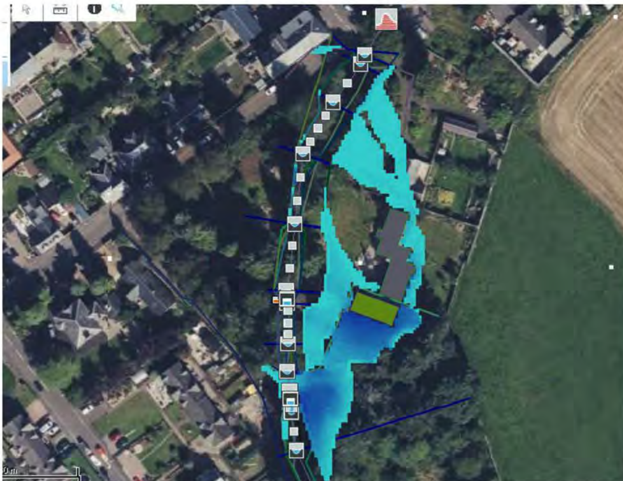
Figure 7 – Predicted 2D 200yr + CC flood extents including 50% of the boundary wall to the east of the watercourse being modelled as solid, and a 25% blockage in the culvert running beneath the driveway of Dalnaglack (MB Error at peak 1D = -0.24%, 2D = 0.5%)
