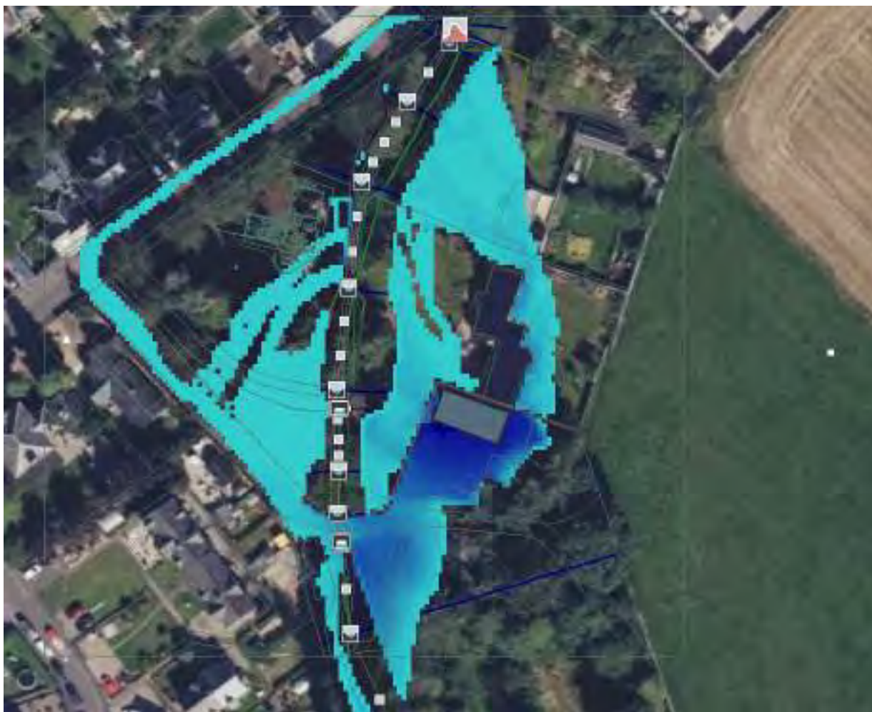
Figure 4 - Predicted 2D 200yr + CC flood extents including 75% of the boundary wall to the east of the watercourse being modelled as solid, and a 75% blockage in the culvert running beneath the driveway of Dalnaglack, with proposed house location overlain.
