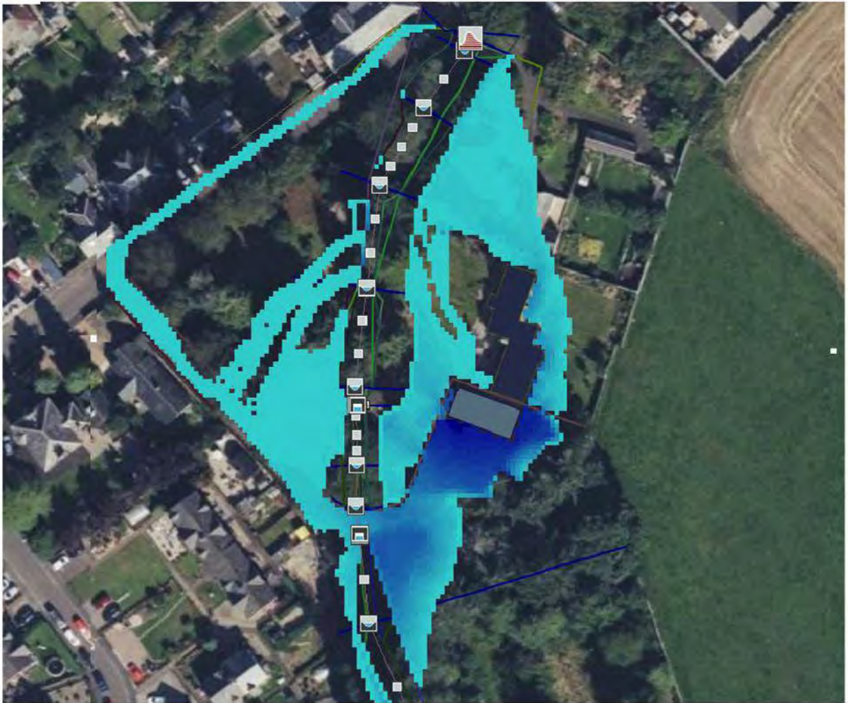
Figure 4 - Predicted 2D 200yr + CC flood extents including 75% of the boundary wall to the east of the watercourse being modelled as solid, and a 75% blockage in the culvert running beneath the driveway of Dalnaglack (MB Error at peak 1D = -0.49%, 2D = 2.2%). Final MB figure in 1D zzd file = 2.83% - please see 1D mass balance summary from zzd file overleaf. Final 2D MB figure = 4.37% - please see 2D mass balance summary overleaf.
