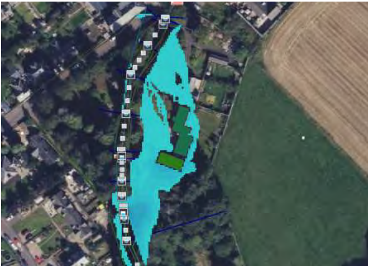
Figure 2 - Predicted 2D 200yr + CC flood extents including a 75% blockage of the culvert running beneath the driveway of Dalnaglack (node Newtyle012.5) (MB Error at peak 1D = -0.51%, 2D = -0.1%)
