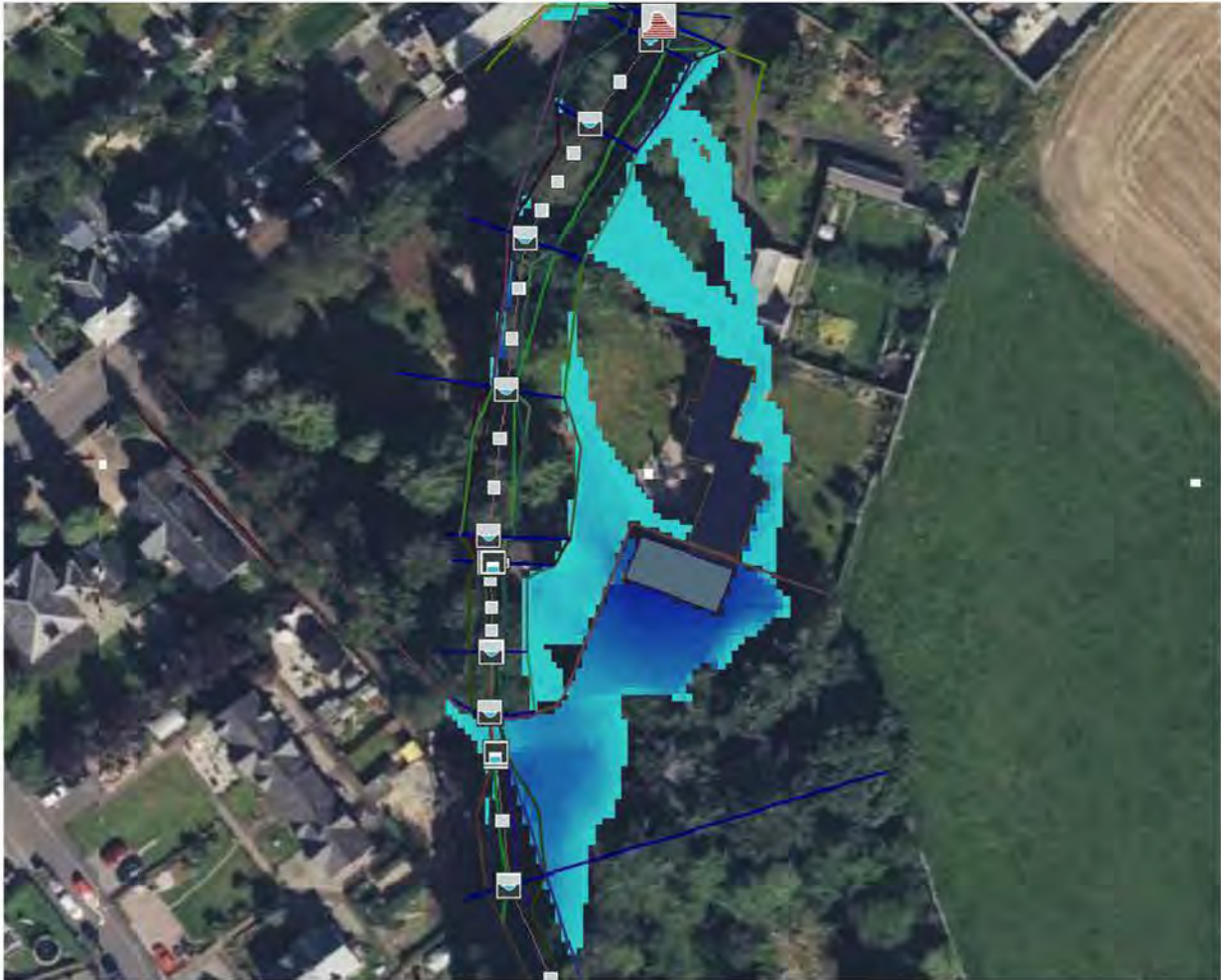
Figure 3 - Predicted 2D 200yr + CC flood extents including 75% of the boundary wall to the east of the watercourse being modelled as solid (MB Error at peak 1D = -0.3%, 2D = -0.7%)
