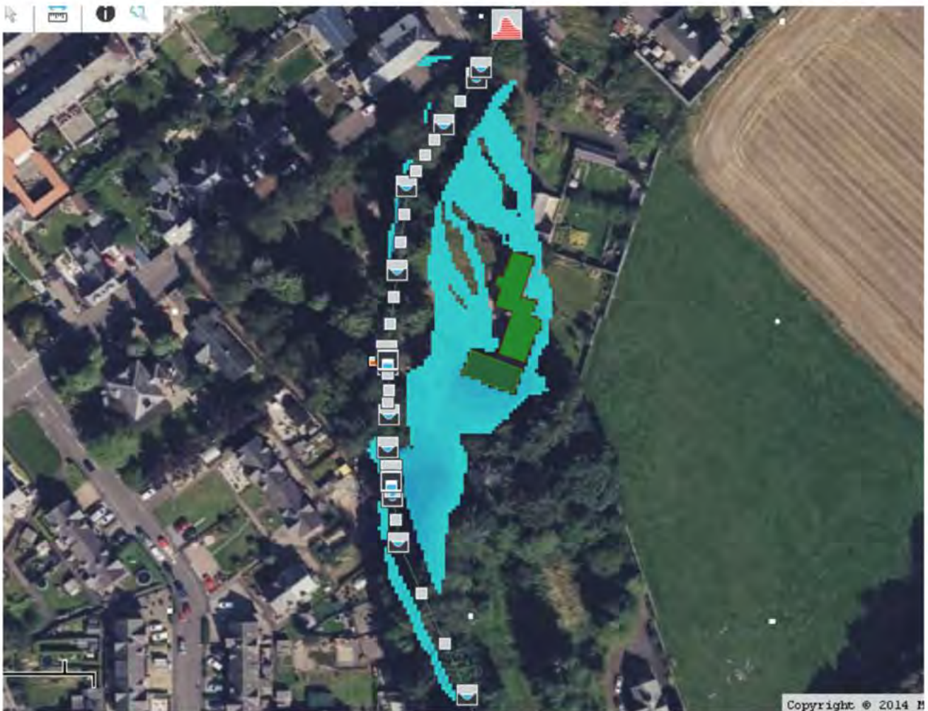
Figure 9 – Predicted 1 in 200yr + CC flood extent from 2D model domain with an increase in roughness of 20%
