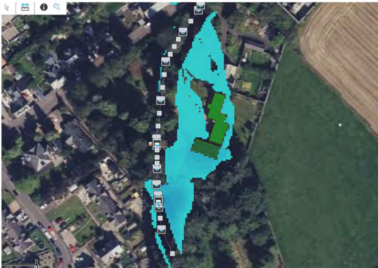
Figure 10 – Predicted 1 in 200yr + CC flood extent from 2D model domain with a 25% reduction in span in the culvert running beneath the driveway of Dalnaglack
