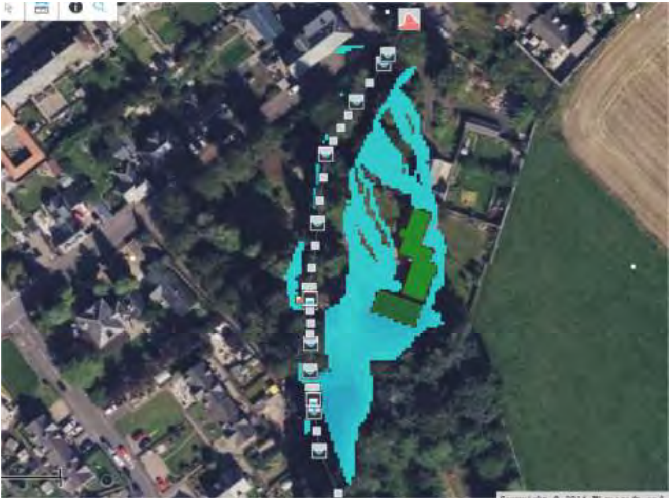
Figure 11 – Predicted 1 in 200yr + CC flood extent from 2D model domain with a 25% reduction in span at the bridge crossing the watercourse at the driveway to Burnbank
